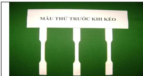
Figure 2.5. Prepare test specimens
