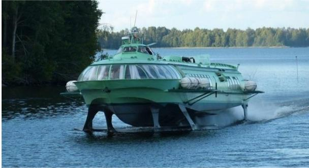
Figure 4.1.a. Hydrofoil ship
